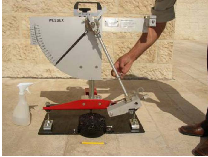
Figure 10 : Modified British Pendulum skid resistance tester.
