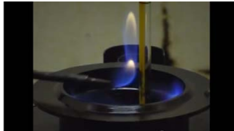
Figure 20 : Flash point test when bitumen start to flash
