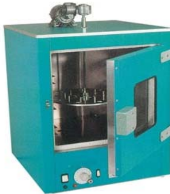
Figure 24: Loss on Heating
