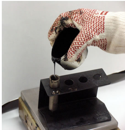
Figure 22 : Pouring a RV sample into the sample chamber.
